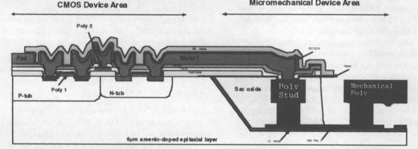
LITTLE INNOVATION, BIG RESULTS — Trench, far right, only microns deep, makes possible fabrication of a wide variety of smart micromachines. Microcircuitry, left, connected directly to micromachine stud, helps make automated control possible by eliminating ghost signals caused by long wiring.
